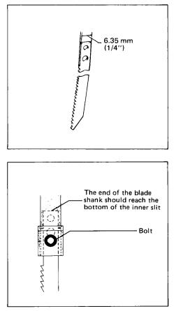
Insert the blade into the blade holder as far as it will go. Make sure that the end of the blade shank reaches the bottom of the inner slit and tighten the bolt securely with the hex wrench.
